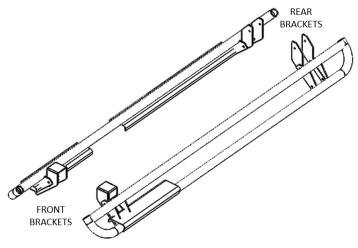
Figure 2. Correct orientation of front and rear brackets assembled.
